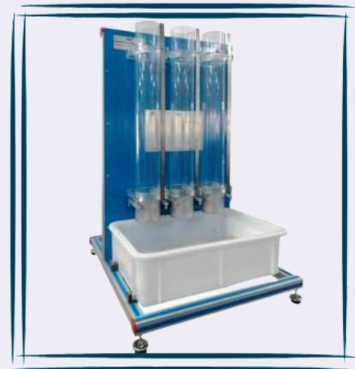
Infiltration Unit (HM 066)
